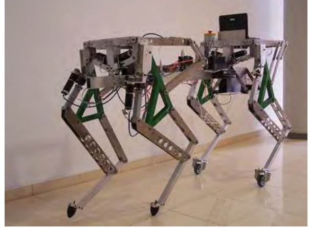
Fig. 12 The hybrid robot including the proposed decoupled leg.
